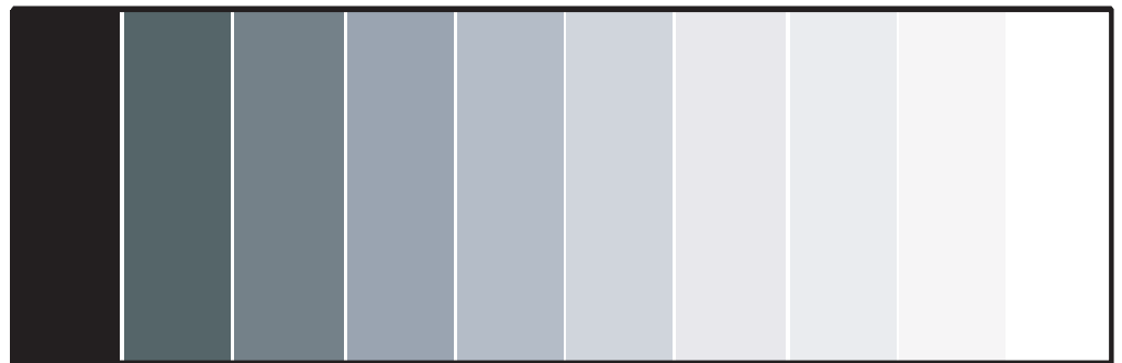
Figure 4-4. Typical Gray Bar Pattern for Adjusting Contrast
